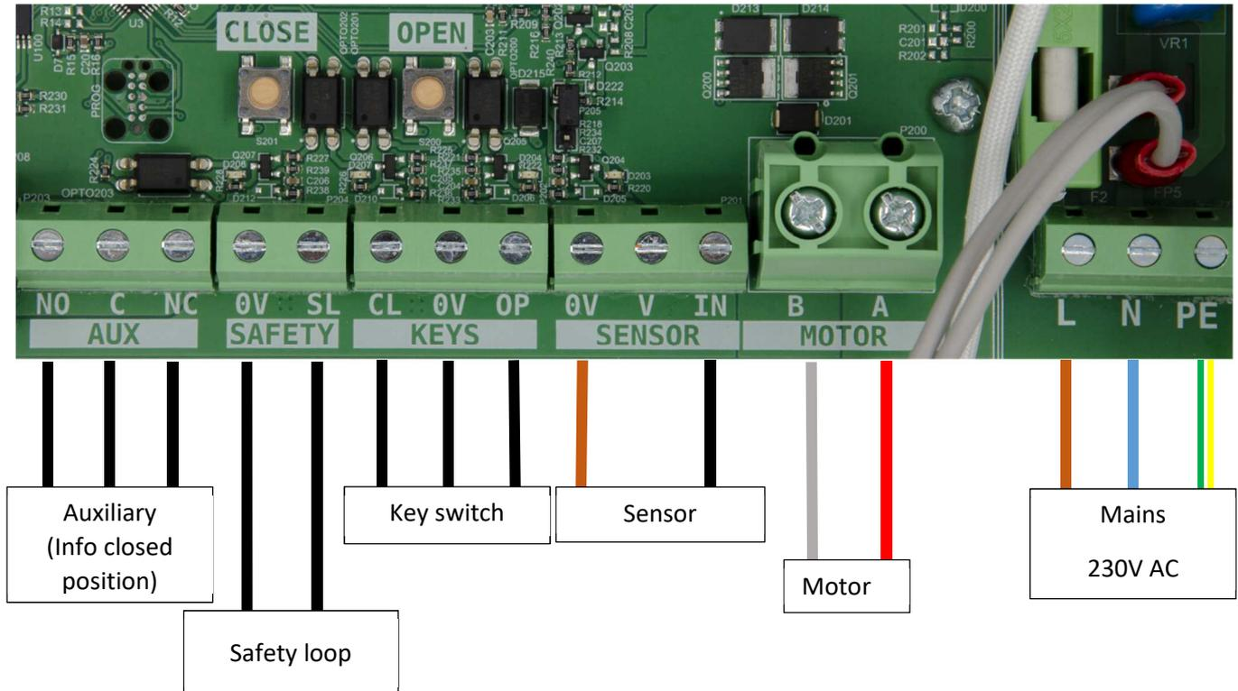
**NOTE:** This wiring schema is valid for a UNICUM motor equipped with mechanical sensor (MLS).
